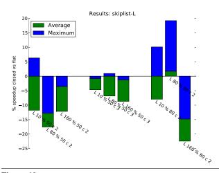
**Figure 10.** Skip-list micro-benchmark. Shows the effect of increasing transaction length. First group contains transactions with 2 calls. For the second group, the number of calls is 3. The last group has 80% reads.
