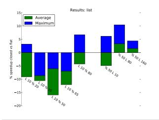
Figure 6. Linked-list micro-benchmark. First group varies read-ratio for short transactions. In the second group, transaction length is varied.
