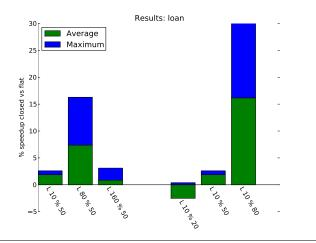
**Figure 5.** Loan monetary application. First group varies transaction length while keeping read-ratio constant. Second group varies the read-ratio for short transactions.
