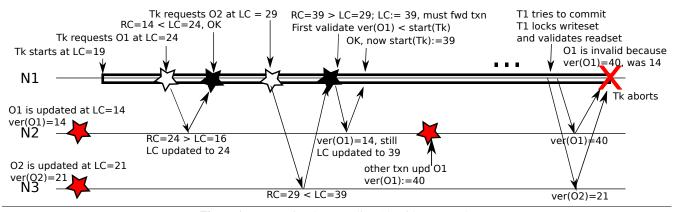
Figure 1. Transactional Forwarding Algorithm Example
