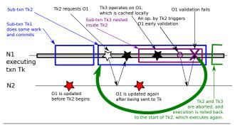
Figure 2. Nested Transactional Forwarding Algorithm Example
