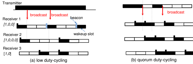
Fig. 1. Opportunistic broadcasting with delivery deferring (a) low duty-cycling case; (b) quorum duty-cycling case with wakeup schedules of [1,1,0,1,0,0,0] and its rotations which comply with (7,3,1) cqs design in [10].
