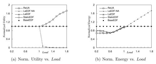
Figure 3: Normalized Energy and Utility vs. Load with Step TUFs under Energy Setting  $E_2$
