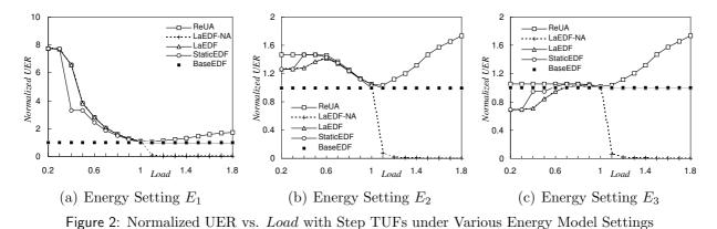
As the figure shows, during overloads, the normalized UERs produced by LaEDF, StaticEDF, and BaseEDF converge to 1. This is because, all three algorithms select the highest frequency by DVS calculation during overloads, and bear no difference in scheduling. As the term  $S_0$  in the energy model increases, ReUA adjusts the selected frequency to accrue more
