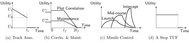
Figure 1: Example Time Constraints Specified Using Time/Utility Functions
